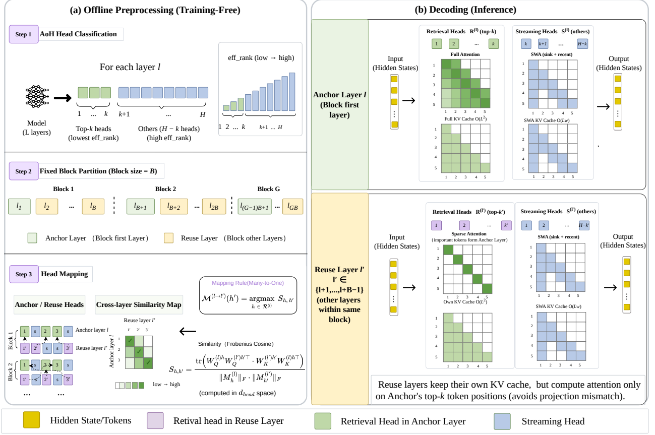
Figure 9: Overview of H2Share. Left: Offline preprocessing classifies heads with AoH, partitions layers into anchor–reuse blocks, and builds cross-layer head mappings. Right: During decoding, anchor retrieval heads compute full attention and select important-token indices; reuse retrieval heads borrow only these indices and attend to their own layer-specific keys and values at the mapped positions; streaming heads use sliding-window attention.
